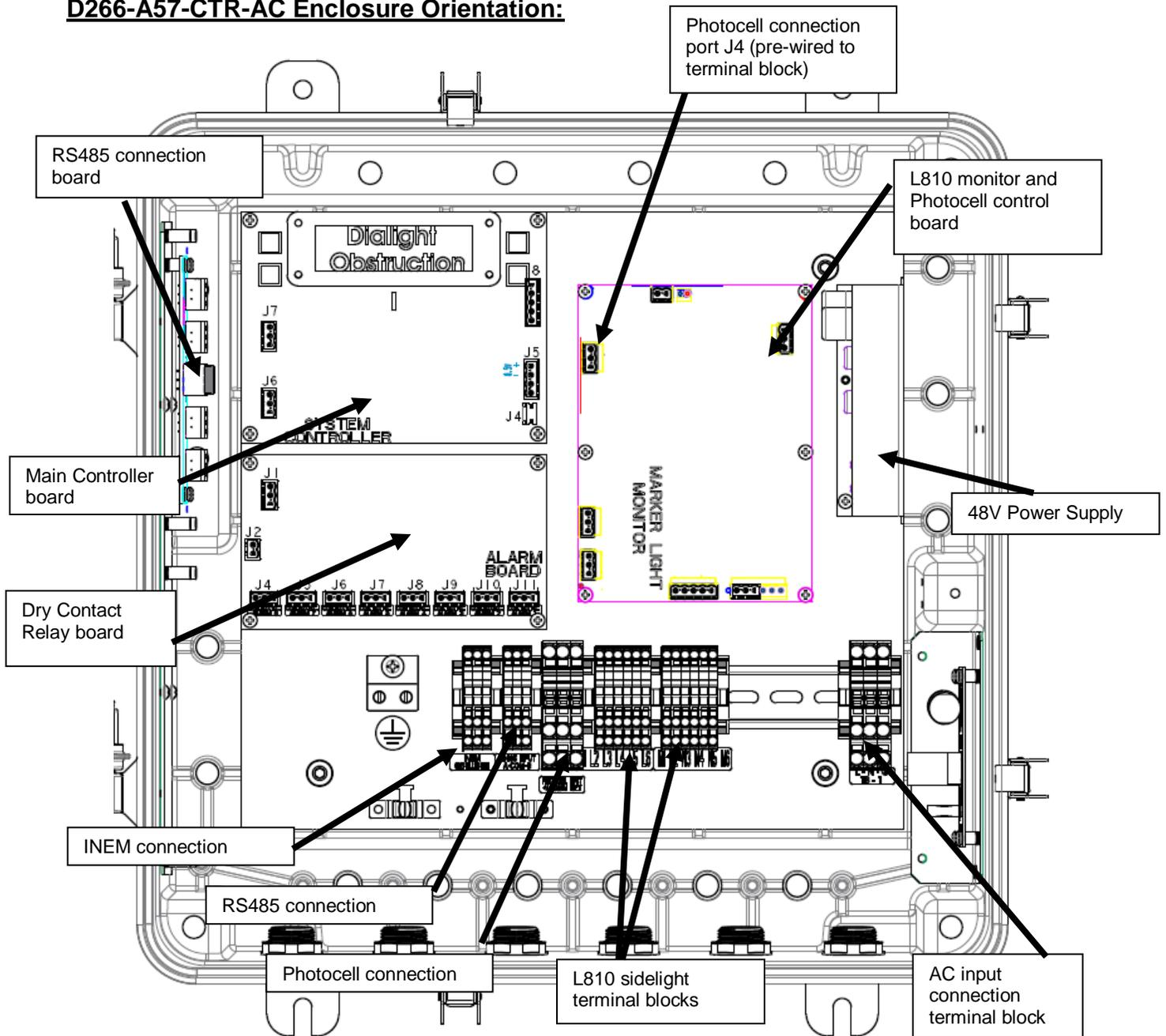
**NOTE:** Multiple grounding points are provided in the enclosure for protective and functional Earth/Ground connections.
