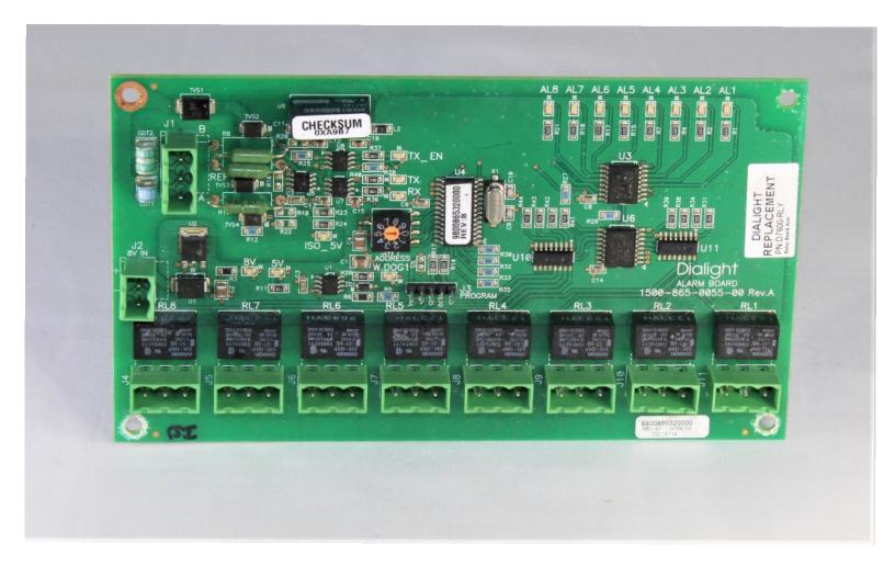
Replacement Alarm Relay Board, D7600-RLY
